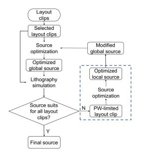
Fig. 1 The conventional final source generation flowchart in real manufacturing.
