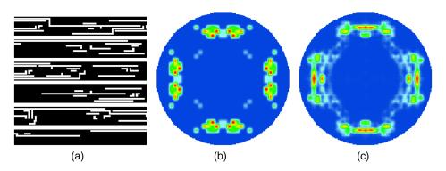
Fig. 8 Illustrations of (a) a layout clip, (b) a model-based source, and (c) an autoencoder-based source.
