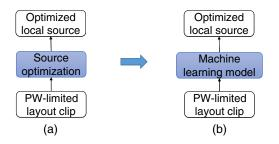
Fig. 2 The comparison of (a) the conventional local source optimization and (b) the autoencoder based source optimization.
