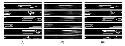
Fig. 9 Illustrations of (a) a layout clip, (b) the reconstruction image of CAE model, and (c) the reconstruction image of U-Net model.
