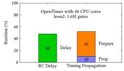
Figure 4: Runtime breakdown for OpenTimer to compute full timing on a million-gate circuit using 40 CPUs [23].
