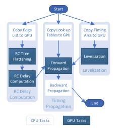
Figure 5: Overall taskflow of the GPU-accelerated STA [23].
