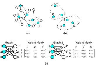
Figure 2: Steps for batch-based independent set matching [13]. (a) Maximal independent set extraction. (b) Independent set partitioning. (c) Batched bipartite matching.
