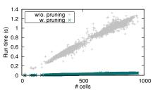
Fig. 2: Pruning speed-up proposed by [30], which can be naturally extended for different metrics, such as wirelength, routability, and congestion.
