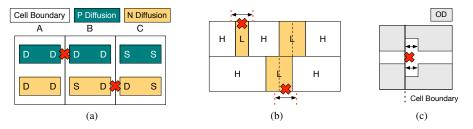
Fig. 3: Example of N10 FEOL rules such as (a) drain-to-drain (D2D) abutment rule and (b) minimum implant area (MinIA) rule and (c) minimum OD jog length (OW) rule.
